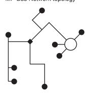
There are no restrictions for the network topology (star, ring, tree or mixed forms are permitted). Supply and communication in one and the same 3-wire cable
